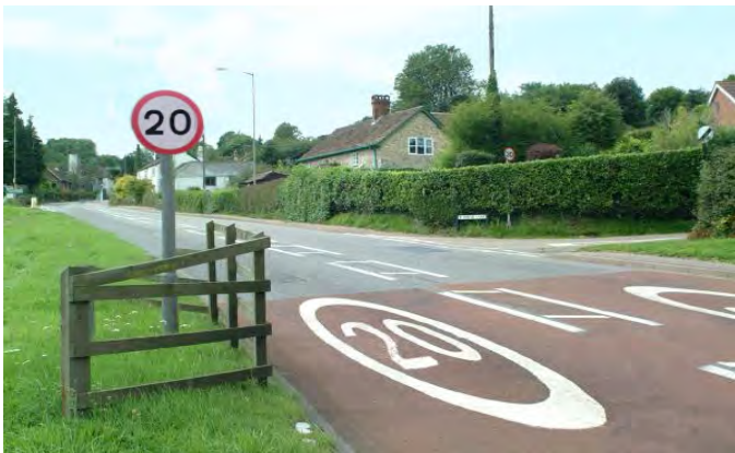
Figure 35: Gateway speed restriction signage
