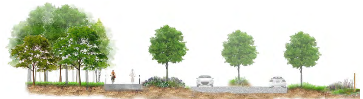
Figure 36: Typical section with carriageways separated by green central reservation area
