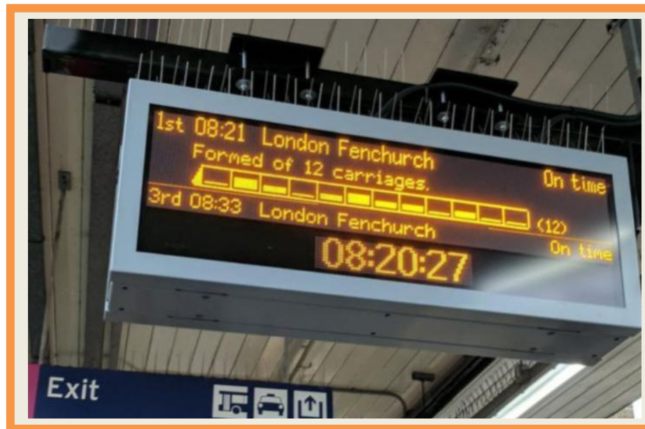
Figure 13: New platform boards showing where likely seating is available on each carriage.
