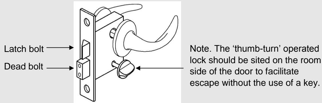
Note. The 'thumb-turn' operated lock should be sited on the room side of the door to facilitate escape without the use of a key.
