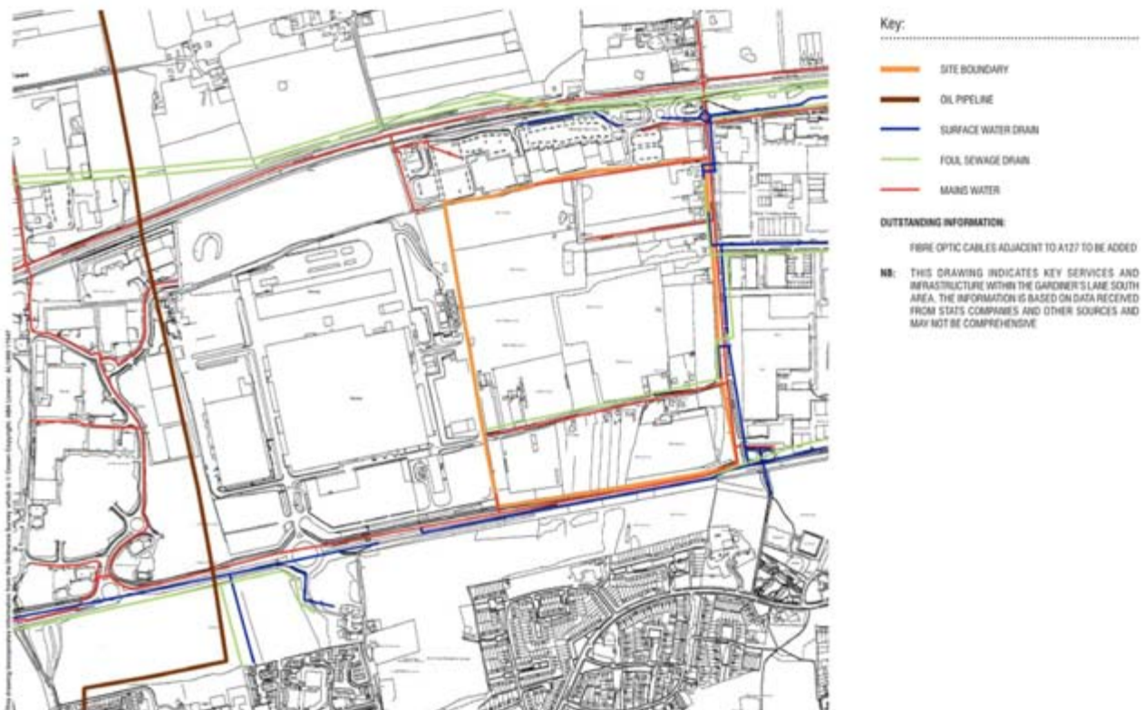
Figure A.3: Existing Services - Surface Water and Drainage
