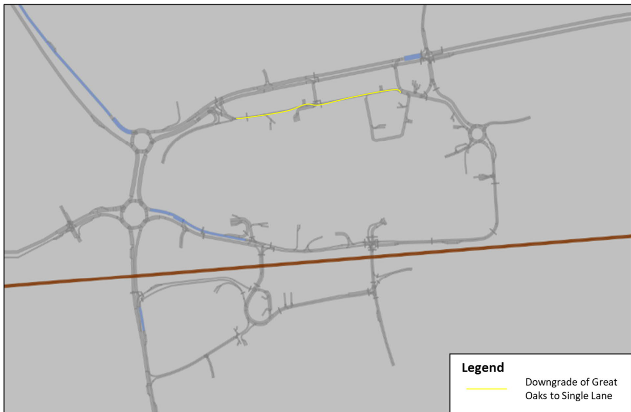
Figure 3.2: Do Something 1 (DS1) Network Link Structure
